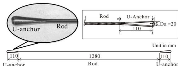
Figure 1 Super CFRP with U-anchor
