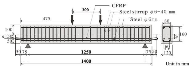
Figure 3 Specimen Detail
