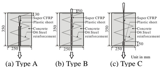
Figure 2 Specimen for Pullout Test
