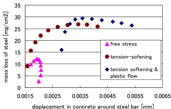
Fig.6 Mass loss of steel and displacement
