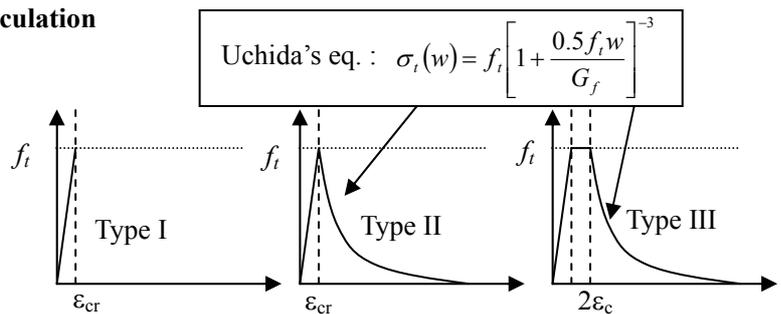
Fig.1 Models of tensile stress of concrete using in calculation
