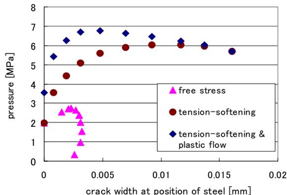
Fig.5 Pressure and crack width at steel position
