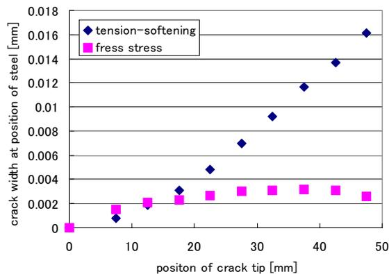
Fig.4 Crack width at steel propagation and crack propagation
