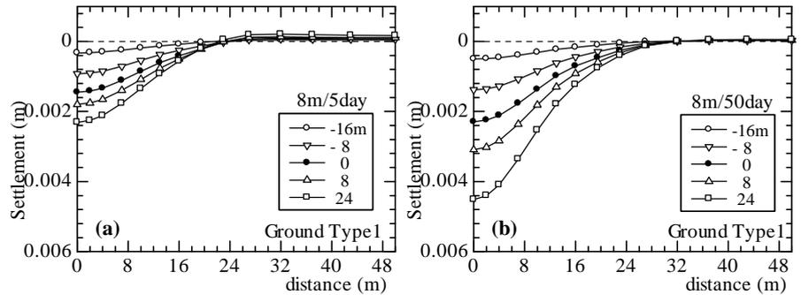
Fig. 4: Surface settlement profiles for ground type 1: (a) Pattern 1; (b) Pattern 2
