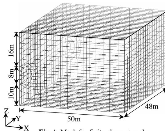
Fig. 1: Mesh for finite element analyses
