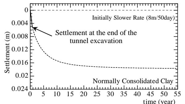
Fig. 8: Surface settlement at the center of the tunnel for ground type 2: Slower rate (up to 55 years)
