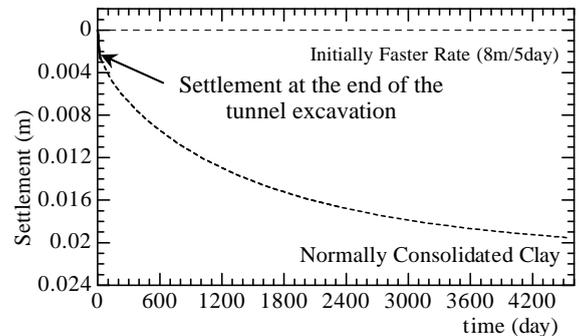
Fig. 6: Surface settlement at the center of the tunnel for ground type 2: Faster rate
