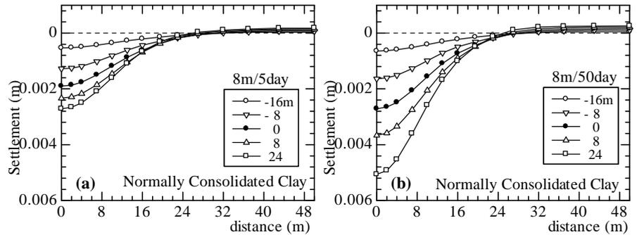
Fig. 5: Surface settlement profiles for ground type 2: (a) Pattern 1; (b) Pattern 2
