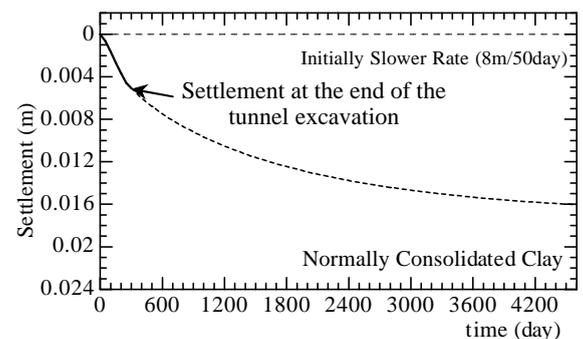
Fig. 7: Surface settlement at the center of the tunnel for ground type 2: Slower rate
