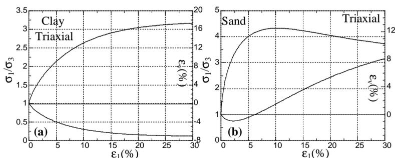
Fig. 3: Stress-strain curves near middle of the ground: (a) Clay; (b) Sand
