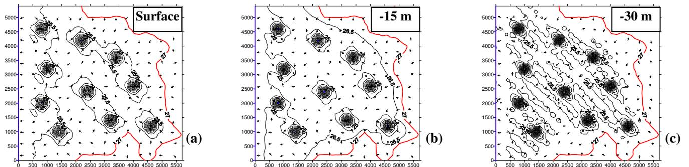
Fig-5 Piezometric Head Distribution of Groundwater Flow under pumping rate 0.01 m<sup>3</sup>/sec from each well
