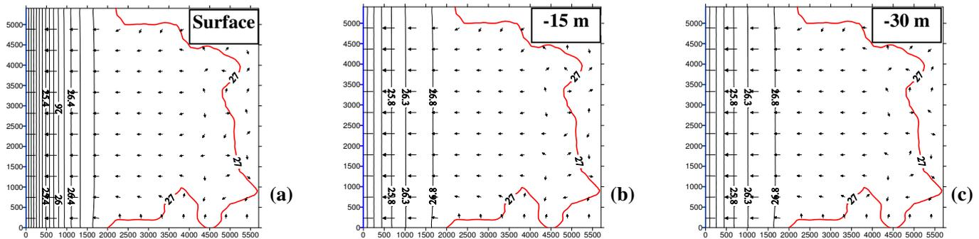
Fig-4 Piezometric Head Distribution of Groundwater Flow under no pumping condition
