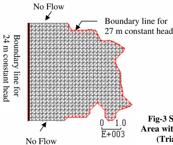
Fig-3 Schematic of Domain Area with Finite Element Grid (Triangular Elements)
