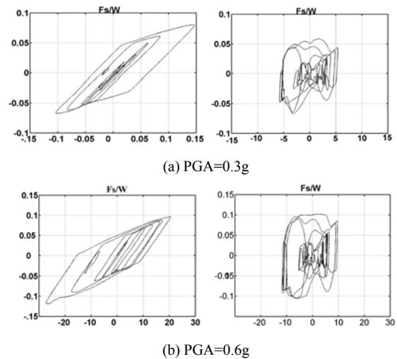
Figure 4. Response of a bilinear model and proposed system under El Centro 1940 ground motion
