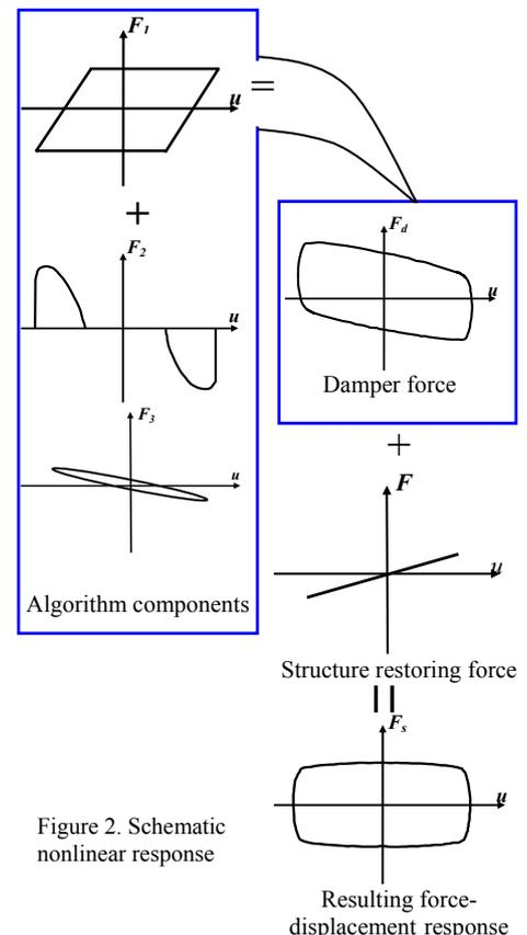
Figure 2. Schematic nonlinear response
