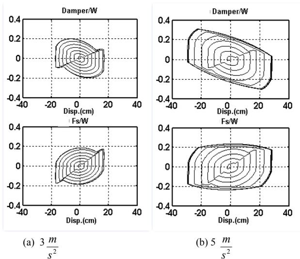
Figure 3. Damper force and Base shear response under resonance harmonic load
