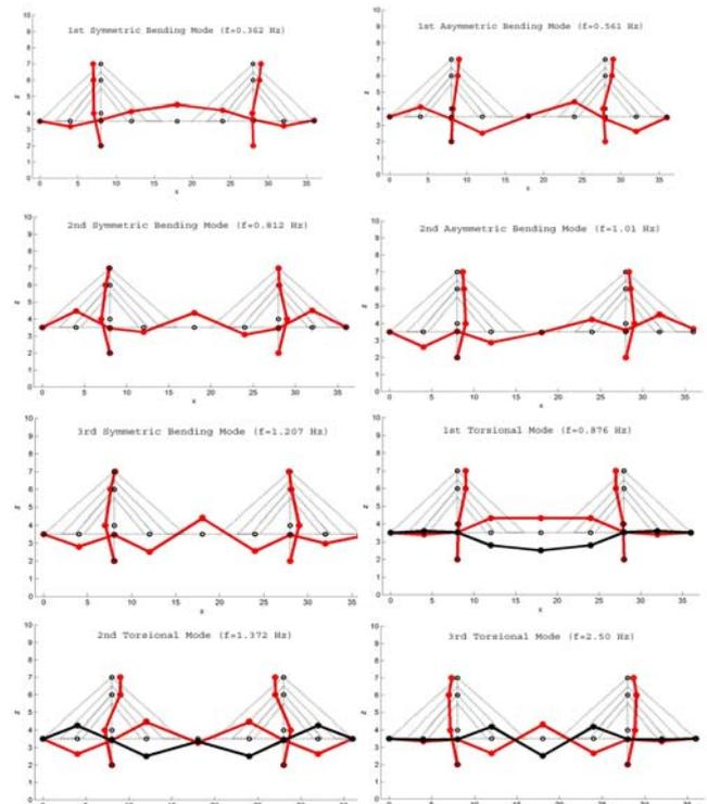
Fig.1: Mode shapes in Longitudinal and Vertical direction
