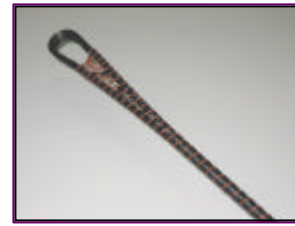
Figure 5 Super-CFRP with U-Anchor
