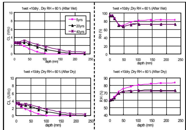
Fig. 4: 1-day wetting and 10-days drying (Drying RH 60%)
