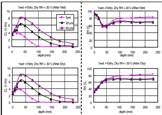
Fig. 3: 1-day wetting and 10-days drying (Drying RH 30%)
