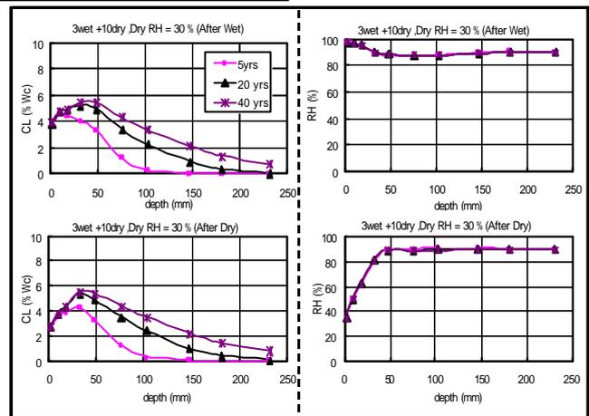
Fig. 2: 3-days wetting and 10-days drying (Drying RH 30%)
