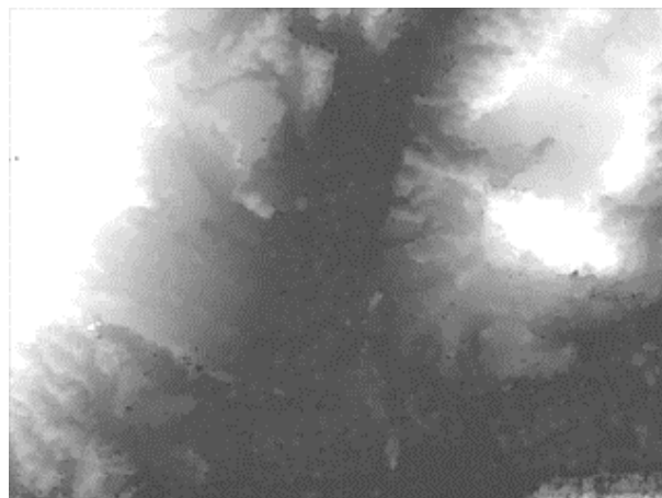
Fig.3 DEM image generated by EROS-A1 stereo pair images
