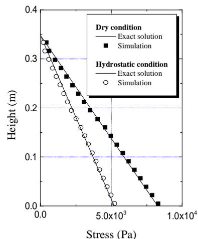
Fig-3 Stress Distribution in y-direction
