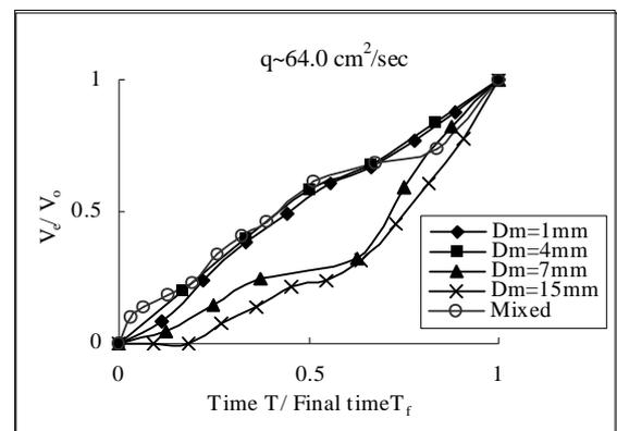
Fig.3 Relationship between  $V_e/V_0$  and  $T/T_f$  in terms of variation in size and composition of dam forming materials
