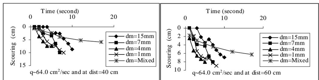
Fig.4 Scouring at particular locations of the dam with time
