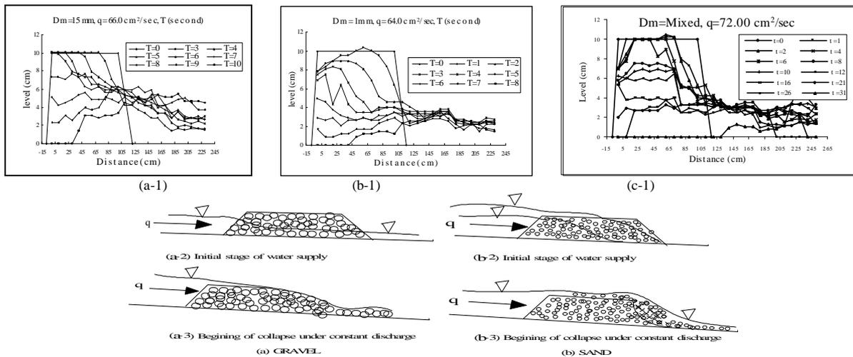
Fig.2 Actual and schematic diagrams of collapse phenomena with the size of dam forming materials
