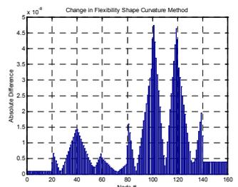
Fig. 7 Change in uniform load curvature method for Case 1
