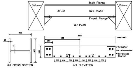
Fig. 1 Actuators and accelerometers position
