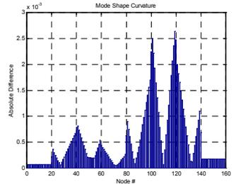
Fig. 5 Mode shape curvature method for Case 1
