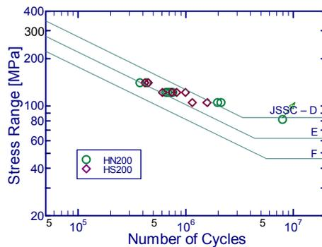
Fig.6 Fatigue test results of H-type specimens
