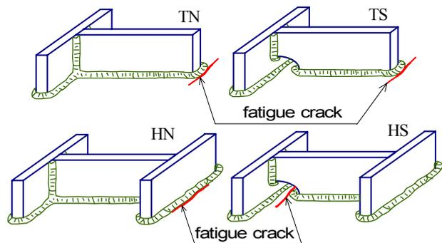
Fig.2 Location of fatigue cracks
