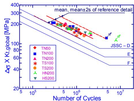
Fig.9 Fatigue test results in terms of 1 mm stress
