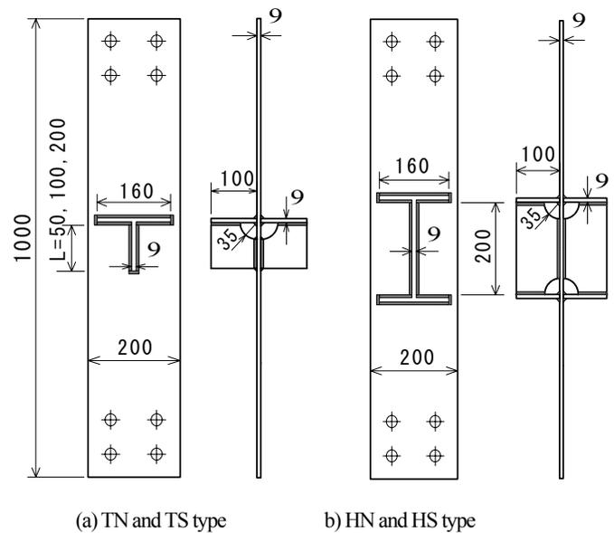
Fig.1 Fatigue test specimens
