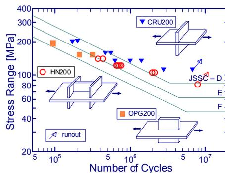
Fig.8 Comparison of fatigue test data of HN200 with cruciform joints and out-of-plane gussets
