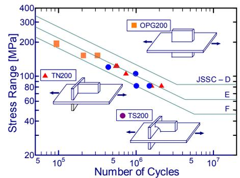
Fig.7 Comparison of fatigue test data of TN200 and TS200 with out-of-plane gussets
