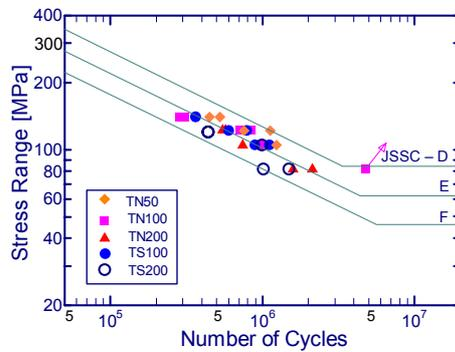
Fig.4 Fatigue test results of T-type specimens
