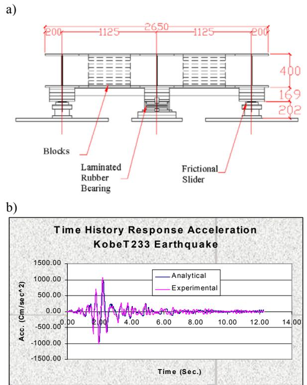
Fig 5- a) Section of Raised Floor
