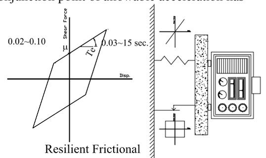
Fig.2- SDOF Resilient Friction Model
