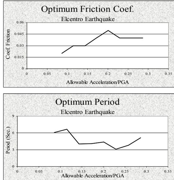
Fig.4- Optimum Parameters for Resilient Friction Model
