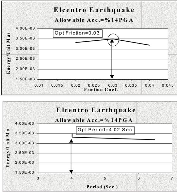
Fig.3- Variation of Dissipated Energy in Resilient Friction Model
