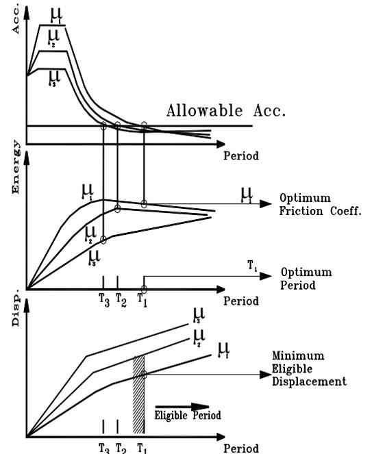
Fig.1- Procedure of optimum parameter recognition
