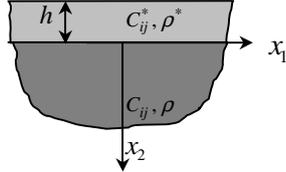
Fig. 1. The anisotropic elastic layered half-space.
