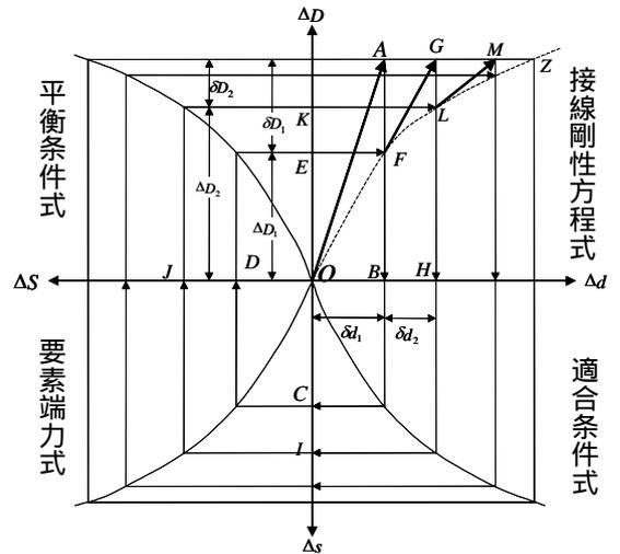
Fig.1 接線剛性法の反復概念
