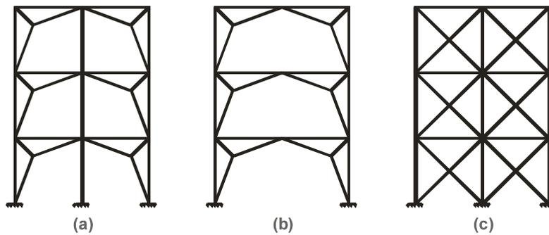
Fig. 1 Frames with Curtain-shape (Y-shape) versus diagonal bracing
