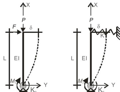
Fig. 4 Model of bracing members
