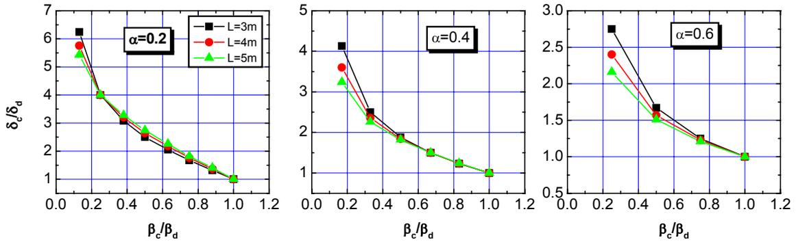
Fig. 3 Lateral displacement ratios of curtain type to diagonal bracing system
