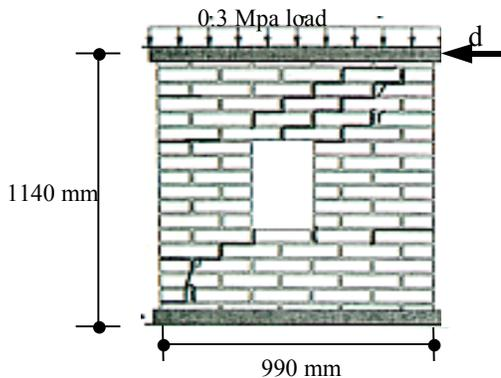
Fig. 4 Experimental crack pattern
