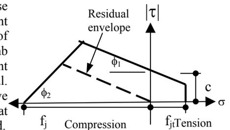
**Fig. 3** Joint failure envelope
