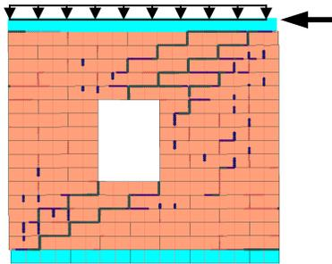
Fig. 5 Crack pattern from numerical analysis
