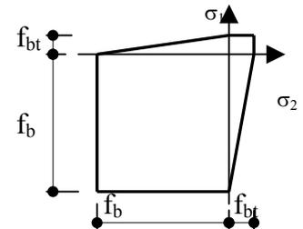
**Fig. 2** Brick unit failure criterion
