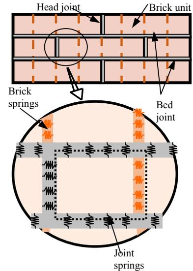
**Fig. 1** Mesh generation Scheme of brick masonry
