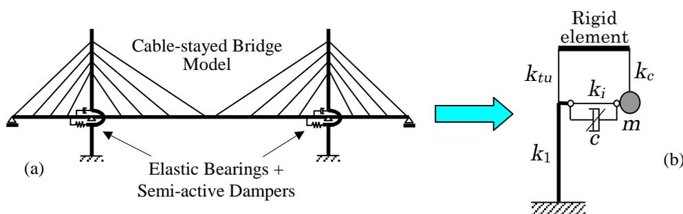
Figure 1. Simplified model for the cable-stayed bridge
