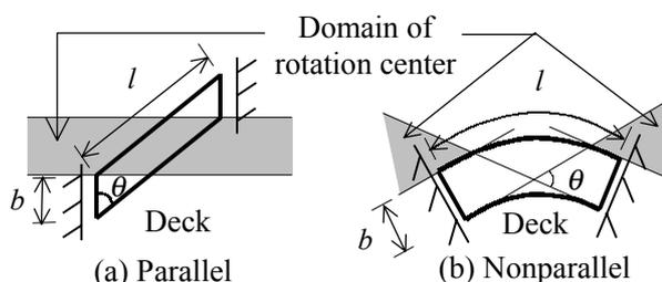
**Fig.1 Domain of center around which the decks can rotate**
