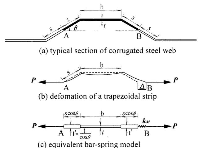
**Fig. 1** Simplified model of corrugated steel web
