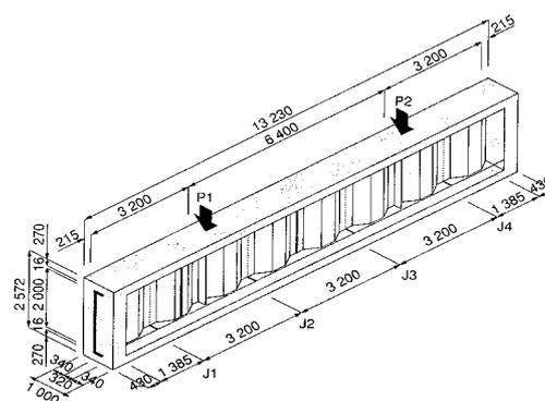
Fig. 3 Test Specimen 1<sup>2)</sup> (in mm)
