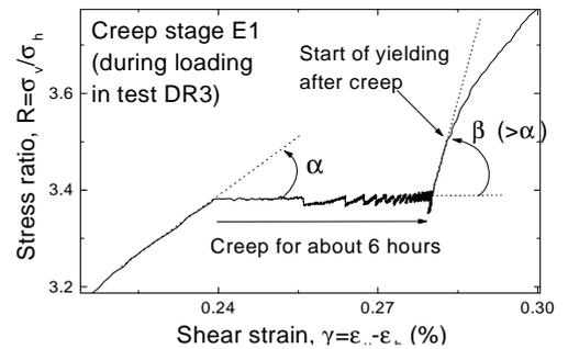
Fig. 5a: Enlargement of creep during stress-loading
