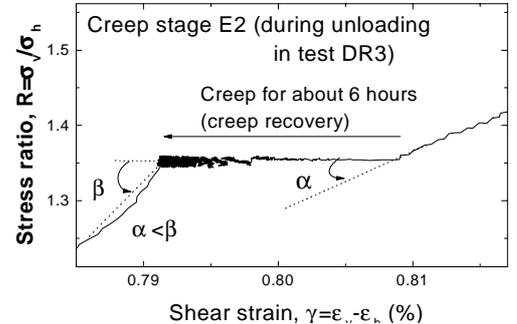
Fig. 5b: Enlargement of creep during stress-unloading
