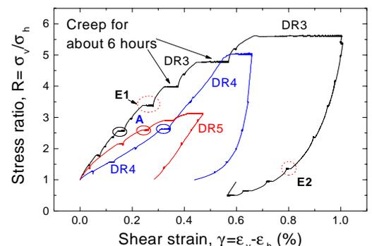
Fig. 3: Stress-strain curves during shearing
