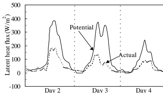
Fig.3. Temporal variations of actual and potential latent heat flux calculated using Penman-Monteith equation
