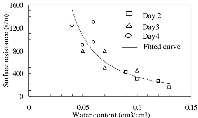
Fig. 5. Variation of soil surface resistance with top 0-1 cm soil moisture
