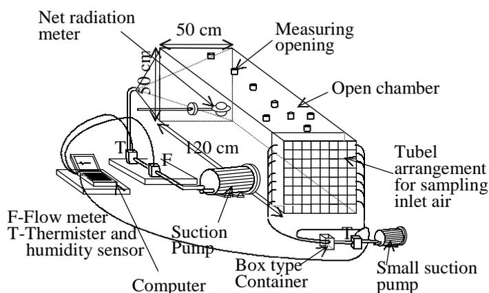
Fig.1 Schematic illustration of the open chamber system for measuring evaporation
