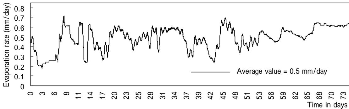
**Fig. 3.** Transient change of the evaporation rate for coarse sand experiment.
