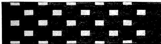
Fig.2 Flow pattern for Type-3 ( Re=10,200 , s=1/60 , F=4.0 )
