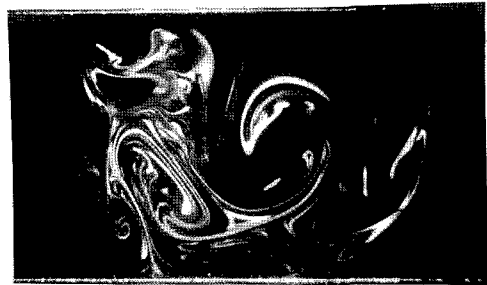
Photo.2 Flow pattern behind cylinder at front view for Type B ( w=60\text{mm} , Re=460 , x=90\text{mm} )
