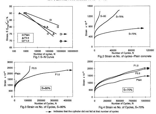
concrete under sustained loading. In the primary portion, strain increases rapidly under cyclic loading. In the secondary portion which consists of most of its life span, strain increases gradually with number of cycles. In the tertiary portion prior to failure, again the strain increases rapidly with number of cycles. The average
