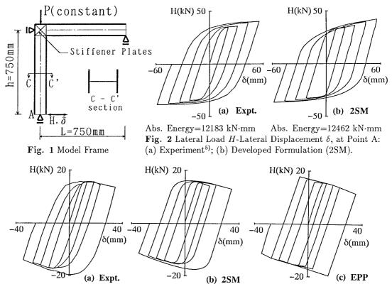
Abs. Energy=3124 kN·mm Abs. Energy=3156 kN·mm Abs. Energy=3224 kN·mm Fig. 3 Lateral Load H-Lateral Displacement  $\delta$ , at Point A: (a) Experiment<sup>5)</sup>; (b) Developed Formulation (2SM); (c) Simplified EPP Moment-Curvature Approach<sup>5)</sup>.
