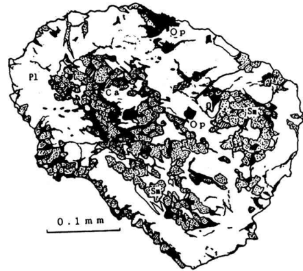
Fig.1 Sketch of Smectite formed in the inner part to zonal structure of Plagioclase phenocryst.
