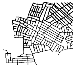
Fig.2 Gas pipeline network of Nankodai
