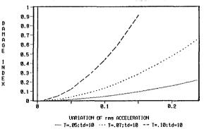
FIG. 1 VARIATION OF D WITH THE rms ACCELERATION (Uu= 8 mm)
