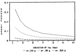
FIG. 2 VARIATION OF D WITH THE MORTAR STRENGTH fmo (td = 10 SEC)
