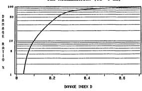
FIG. 3 DAMAGE RATIO (%) SCALE IN TERMS OF THE DAMAGE INDEX D
