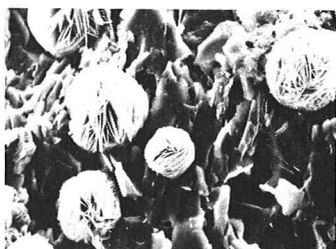
写真-6 変成安山岩 (0.1 N NaOH 48 h )
