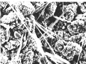
写真-8 輝石安山岩 (1 N NaOH 48 h )
