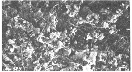
Fig. 4b SEM micrograph of biofilm on sample 3 (1st tank)
