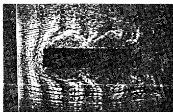
Photo. Flow around Rectangular cross section Fixed at incidence angle of \varphi=0^\circ Pulsating flow with f_p=2f_s
