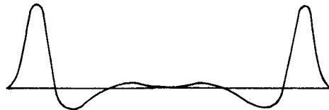
Gross buckling failure mode
