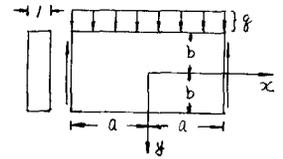
$$y = -b; \quad \sigma_y = -q, \quad \tau_{xy} = 0, \quad y = +b; \quad \sigma_y = \tau_{xy} = 0. \quad (1-a)$$
