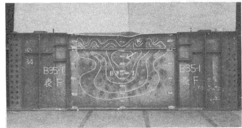
Photo 2 Collapse Mode of Test Panel (B-35-1)
