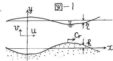
$$\text{河床面において: } \frac{\partial \psi}{\partial x} = \frac{dh}{dt} \quad \dots \dots (10), \quad u_*^2 = \frac{(\bar{u}_b - C_r)^2}{\{1.9 + 2.5 \ln(D_{fs})\}^2} \quad \dots \dots (11)$$
