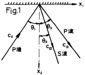
$$\left. \begin{aligned} \phi^{(r)} &= \frac{A}{ZP} \left( t - \frac{x_1 \sin \theta_3 + x_2 \cos \theta_3}{C_{12}} \right)^2 H\left(t - \frac{x_1 \sin \theta_3 + x_2 \cos \theta_3}{C_{12}}\right) \\ \psi^{(r)} &= \frac{B}{ZP} \left( t - \frac{x_1 \sin \theta_2 + x_2 \cos \theta_2}{C_{22}} \right)^2 H\left(t - \frac{x_1 \sin \theta_2 + x_2 \cos \theta_2}{C_{22}}\right) \end{aligned} \right\} \quad (11)$$
