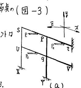
部材角モーメント;  $(M_R^k)_{P1} = (\tilde{M}_R^k)_{P1}$ ,  $(M_R^k)_P = (\tilde{M}_R^k)_P + (C_R^k)_P A_0$ ,  $(M_R^k)_{P1} = (\tilde{M}_R^k)_{P1}$ , 又  $M_P = -\frac{1}{3}(C_R^k)_P A_0$  (図-3)
