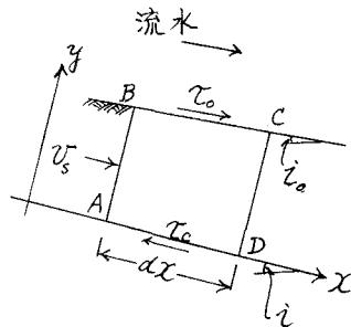
$$F_{p1} - F_{p2} = -\frac{\partial}{\partial x} (b \delta (p + \frac{P_g g}{2} \delta)) dx, F_w = \delta (p + \frac{P_g g}{2} \delta) \frac{db}{dx} dx, F_c = p b \frac{\partial \delta}{\partial x} dx, F_g = \rho_s g b \delta i_o dx$$
