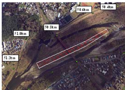
Photo 4 The area of bed excavation (a pilot channel) over the forested bar
