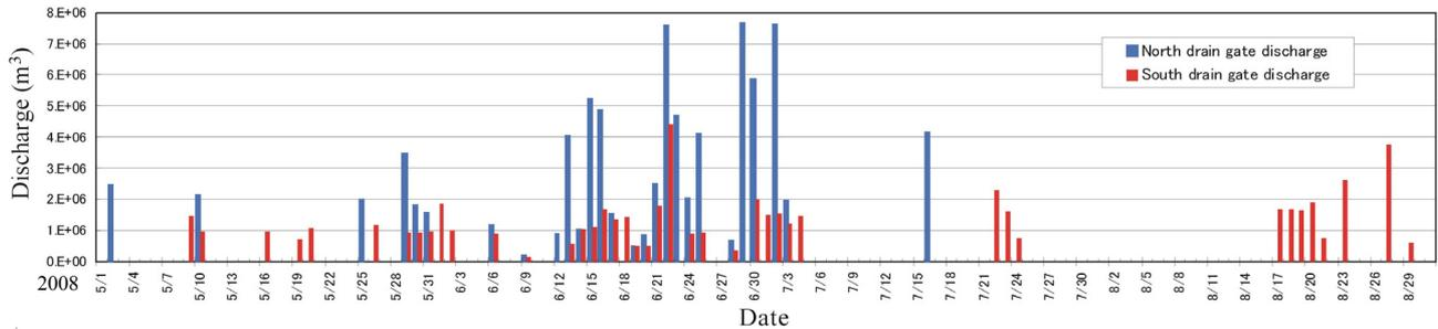
**Fig.3** Discharge of the north drain gate and the south drain gate.
