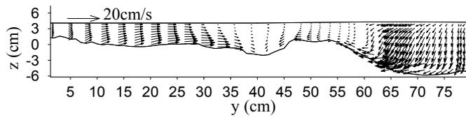
**Fig.10b** Flow velocity (v, w) at x=-22cm (Sim.).
