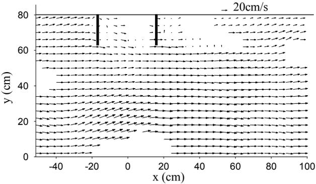
**Fig.9a** Flow velocity (u, v) at 2cm from initial bed (Exp.).
