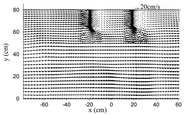
**Fig.8b** Flow velocity (u, v) on water surface (Sim.).
