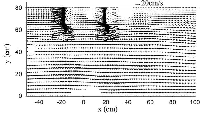
**Fig.9b** Flow velocity (u, v) at 2cm from initial bed (Sim.).
