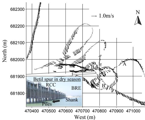
Fig.2 Flow velocity ( $u, v$ ) near water surface.
