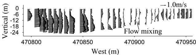
Fig.3 Flow velocity ( $v, w$ ) in vertical plane A-A.
