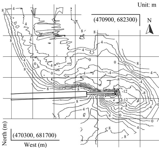
Fig.1 Bed bathymetry around Betil spur (July 19, 2008).
