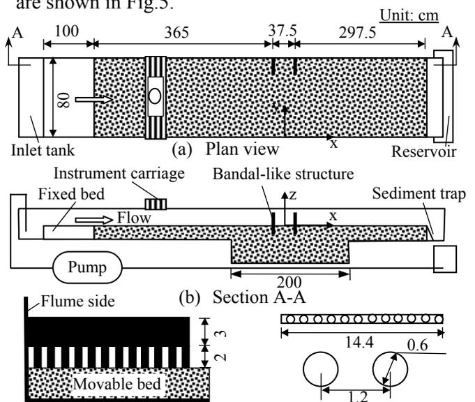
(c) Bandal-like structure: side view, top view and piles details
