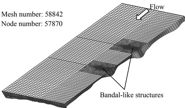
**Fig.7** Computational mesh around Bandal-like structures.
