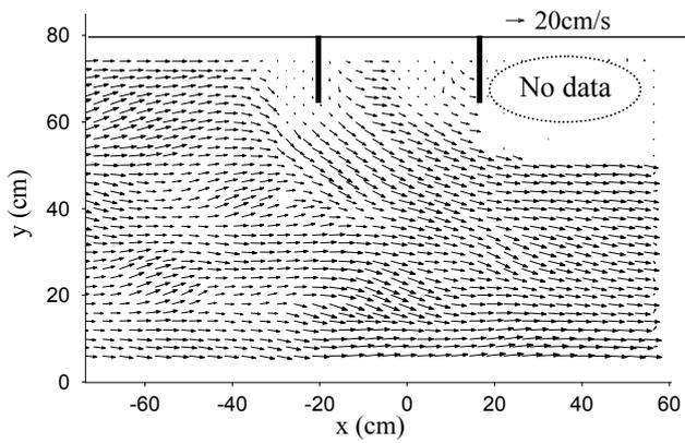
**Fig.8a** Flow velocity (u, v) on water surface (PIV).
