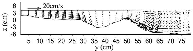
**Fig.11b** Flow velocity (v, w) at x=-16cm (Sim.).
