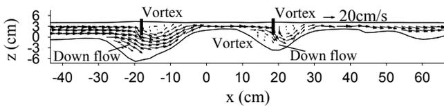
**Fig.12a** Flow velocity (u, w) at y=72cm (Exp.).
