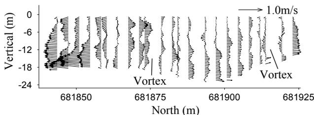
Fig.4 Flow velocity ( $u, w$ ) in vertical plane B-B.
