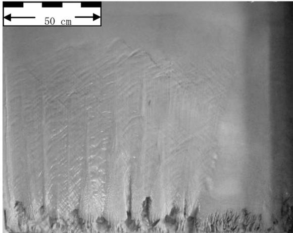
**Fig. 5** Channelization process by pure surface erosion.
