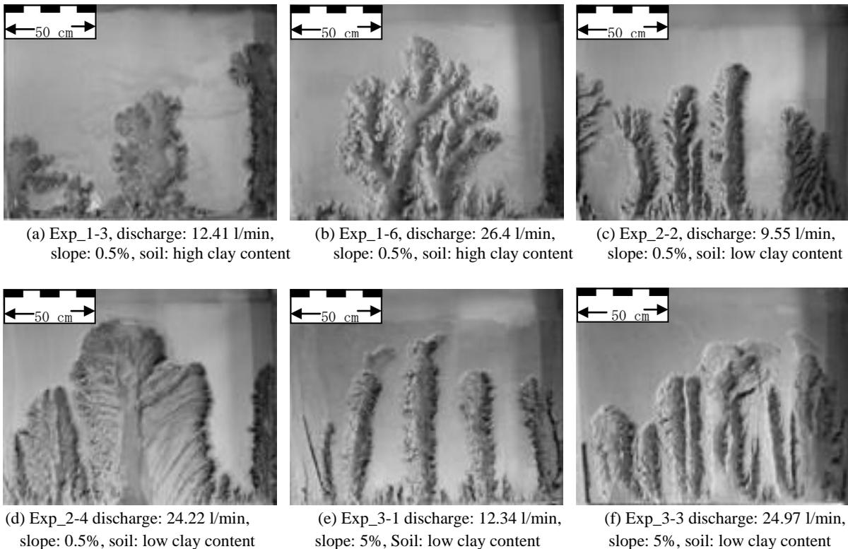
**Fig. 6** An over view of the experiments: (a) and (b) are experiments conducted with high clay content (first series); (c) and (d) are experimental pictures among soils with low clay content and mild slope (second series); and (e) and (f) are among experiments with less clay content but steep slope (third series).
