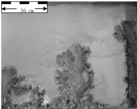
Fig. 2 Channelization process by undercutting and mass failure.
