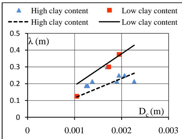
Fig. 7 Channel spacing versus Froude-critical depth for the experiments conducted in mild slope. The solid line represents regression equation for both sediment mixtures.
