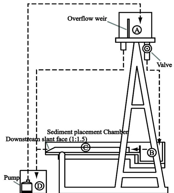
Fig.1 Experimental apparatus: the broken line indicates water flow path. A: discharge head regulator; B: water collector chamber; C: sediment placement chamber; D: reservoir
