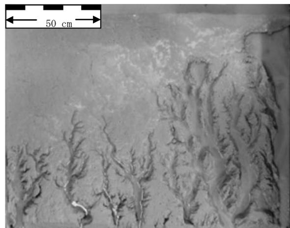
Fig. 4 Channelization process by localized erosion.
