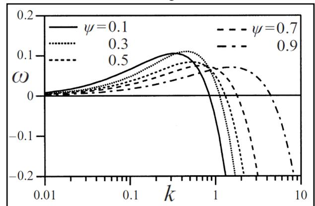
Fig. 8 Dependency of  $\omega$  on  $\psi$  and  $k$ , for  $\sigma = 0$  &  $\gamma = 1.5$ : adopted from Izumi and Parker<sup>1)</sup>.
