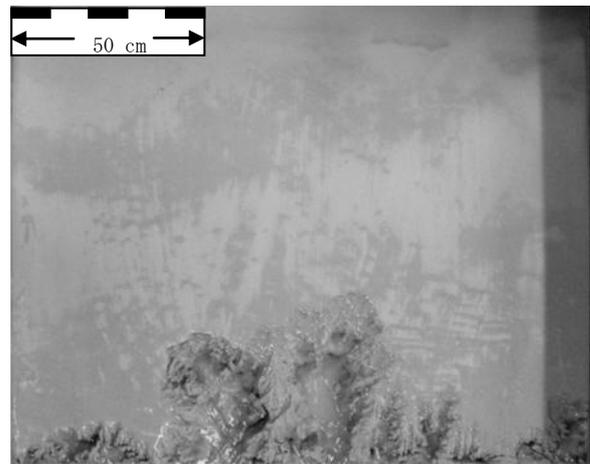
Fig. 3 Channelization by undercut and mass failure preceded by erosion.
