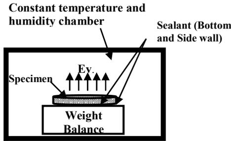
Fig. 3 Experimental condition for the measurements of evaporation from a rock specimen (Maung, *et al.*).
