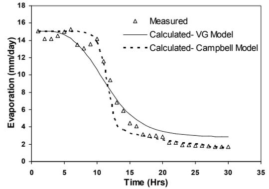
Fig. 6 Measured and calculated evaporation for sedimentary rock.
