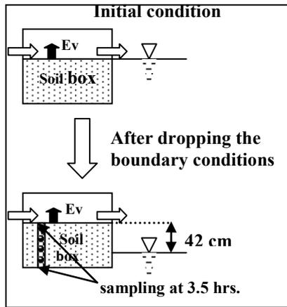
Fig. 5 Procedure of the experiment.
