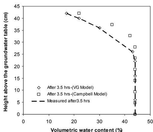
Fig. 11 Comparison between measured and calculated water contents for fine sand.
