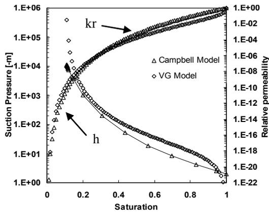
Fig. 8 Estimated hydraulic functions of sedimentary rock.
