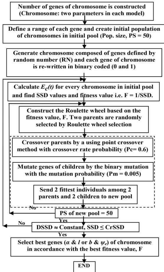
Fig. 2 Flow chart of GA application in the inverse solution.
