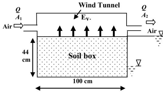
Fig. 4 Schematic view of evaporation measurement equipment.
