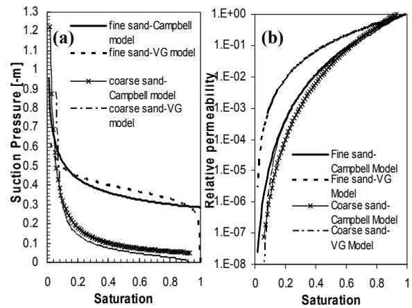
Fig. 10 Estimated hydraulic functions of soils.
