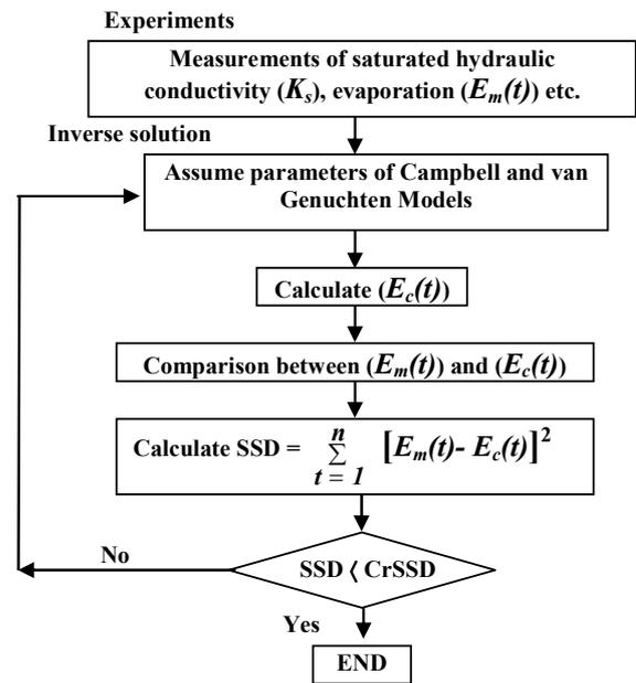
Fig. 1 Procedure of the inverse solution technique.
