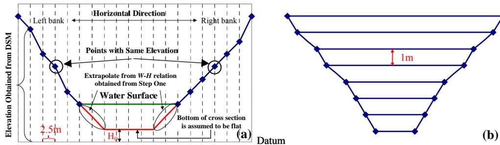
**Fig. 1 (a)** The schematic description of deriving relation between cross-sectional width and corresponding elevation from DSM data. **(b)** The geometrical model describing cross-section shape which consists of a series of symmetrical trapezoids
