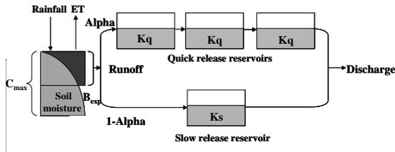
**Fig.3** Schematic description of HYMOD's structure
