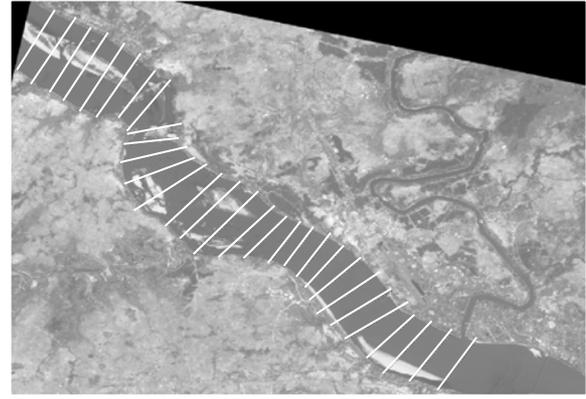
**Fig.4** Locations of 30 cross-sections at Pakse for which  $W-H$  relation is measured from DSM
