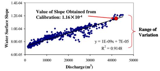
**Fig.7** Relation between observed discharge and water surface slope at Pakse region
