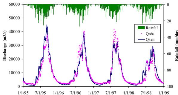
**Fig.6** Observed and simulated discharge for 1995-1998
