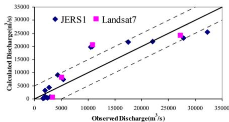
**Fig.8** Estimated discharge plotted against observed discharge based on Eq.(3) for width records derived from 16 scenes of JERS-1 images and 4 scenes of Landsat7 images
