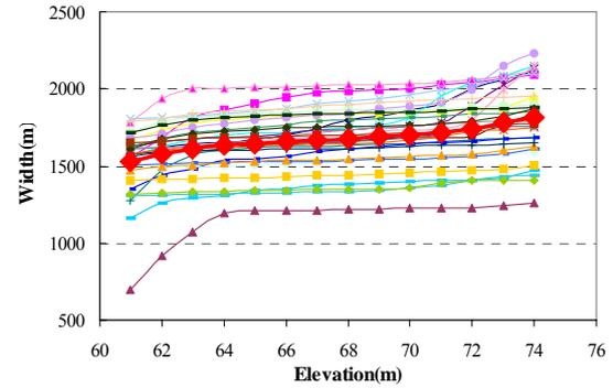
**Fig.5** The derived  $W-H$  relations for the 30 cross-section and the average relation (thick red one)
