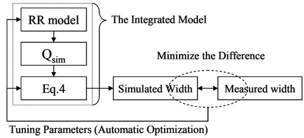
**Fig.2** The integrated model and calibration scheme
