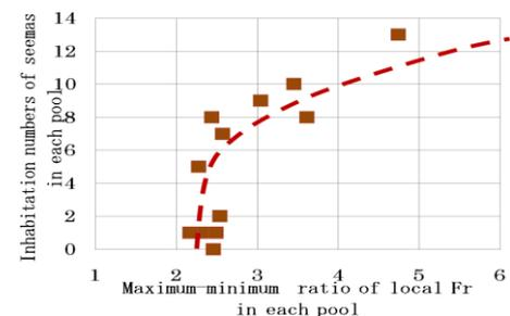
**Fig.11** Relation between maximum-minimum ratio of local Froude number in each pool and the number of masu salmon inhabiting the pool.
