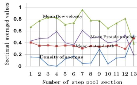
**Fig.10** Sectional averaged hydraulic values in each pool.
