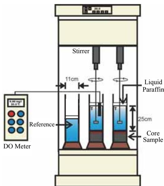
**Fig.3** Experimental set-up for SOC measurements.
