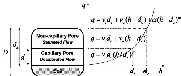
**Fig. 1** Schematic model structure and extended stage-discharge relationship of OHDIS-KWMSS.
